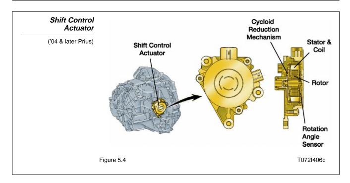
**SERVICE TIP** If there is a malfunction in the shift control actuator, the vehicle will not go into park. The Master Warning Light will illuminate, the shift position indicators on the dash will flash, and the Park button light will flash.
