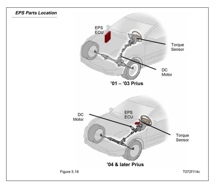
**EPS ECU** The EPS ECU uses signals from the torque sensor to interpret the diver's steering intentions. It combines this information with data from other sensors regarding current vehicle conditions to determine the amount of steering assist that will be required. It can then control the current to the DC motor that provides steering assist current to the DC motor that provides steering assist.
