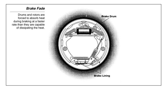
Lining fade affects both drum and disc brakes and occurs when the friction material overheats to the point where the coefficient of friction drops off. When the coefficient of friction drops off, friction is reduced and the brake assemblies ability to convert added heat is reduced.
