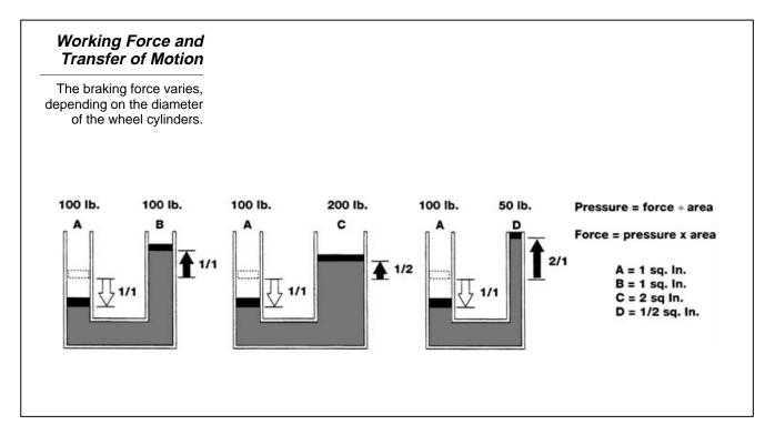
Hydraulic brakes deliver equal braking force to all wheels with a minimum of transmission loss. Hydraulic brakes have a wide design flexibility because braking force can be changed merely by changing the diameter of the master cylinder and wheel cylinders.
