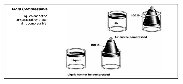
Fluid pressure is indicated in pounds per square inch (psi). It is determined by dividing the input force applied to a piston by the area of the piston. (force/area = pressure in psi) If a force of 100 pounds is applied to a master cylinder piston, an area of 2 square inches, the resulting pressure will be 50 psi. This pressure is transmitted to all parts of the fluid in the container equally.
