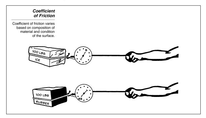
The following example illustrates how the type of friction surface can influence the coefficient of friction (COF).
