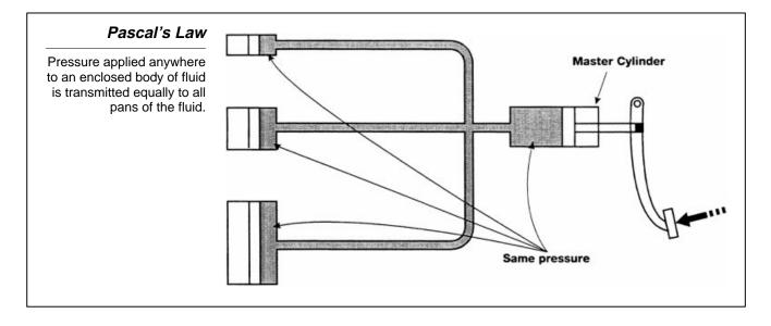
Another important distinction to make is that liquids cannot be compressed, whereas, air is compressible. A hydraulic system must be free of air in order to function properly. Pedal travel will increase as air in the system is compressed.
