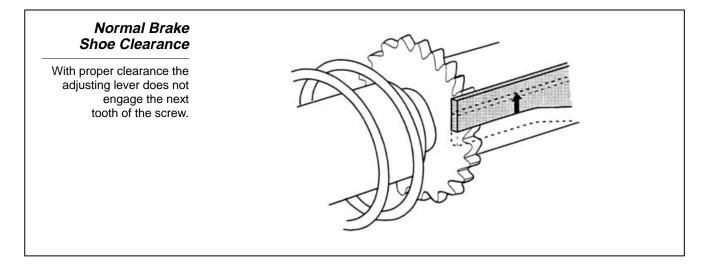
The adjusting lever is arranged in such a way as to engage with one adjusting screw tooth. Therefore, one operation of the parking brake lever only advances the adjusting screw by one tooth, reducing brake shoe clearance by approximately 0.012" (0.03mm), even when there is a large amount of brake shoe clearance.
