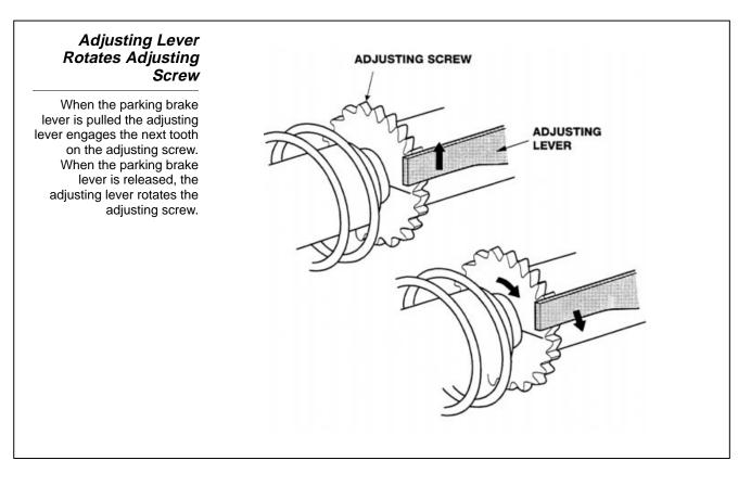
When the brake shoe clearance is normal and the parking brake lever is pulled, the adjusting lever moves only a small distance. The adjusting lever does not move to the next tooth of the adjusting screw. Brake shoe clearance remains unchanged as a result.
