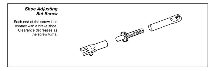
Since each end of the adjusting screw is in contact with a brake shoe, the brake shoe clearance decreases as the screw turns.
