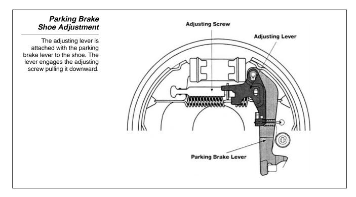
When brake shoe clearance is greater than standard and the parking brake lever is pulled, the adjusting lever moves over to the next tooth of the adjusting screw.
