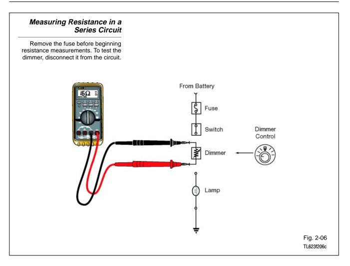
**Resistance in a series circuit -** To make resistance measurements:
