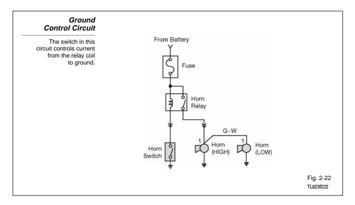
**Ground control -** The horn circuit shown here is an example of a ground control circuit.
