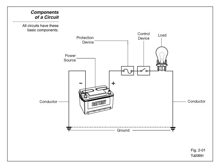
**Power source -** In automotive circuits, the source is typically the battery.
