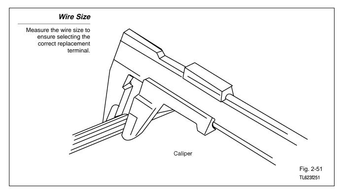
5. Select the correct replacement terminal, with lead, from the repair kit.
