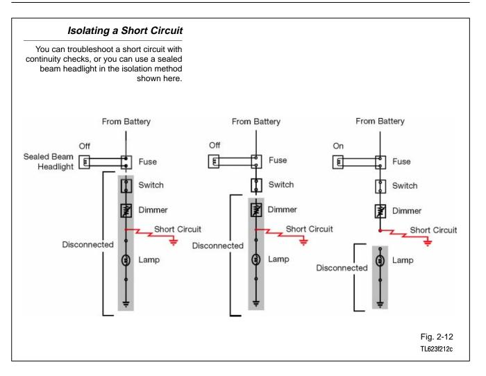
**Isolating a short circuit -** Circuit breakers and short detectors may damage some circuits. The following method works well for locating most short circuits:
