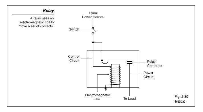
**Relay** - A relay functions as a remote-control switch. It uses a small current to control a larger current. A typical application for a relay is to control a load that requires a large current with a switch that controls a small current. Using a relay for remote switching has these advantages:
