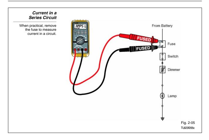
**Current in a series circuit -** Current in a series circuit is the same at every point in the circuit.
