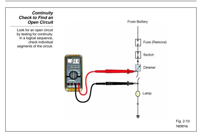
**Testing for continuity -** The preferred method of testing a circuit is with power applied and checking for voltage drop.
