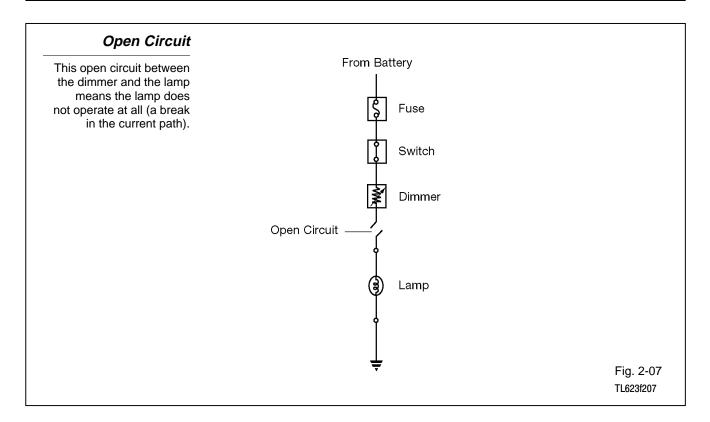
**Open circuit** - Any break (open) in the current path of a series circuit makes the whole circuit inoperative. Open circuits can be caused by:
