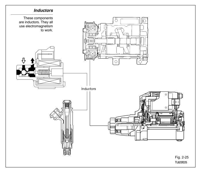
Solenoids, relays, motors, and coils:
