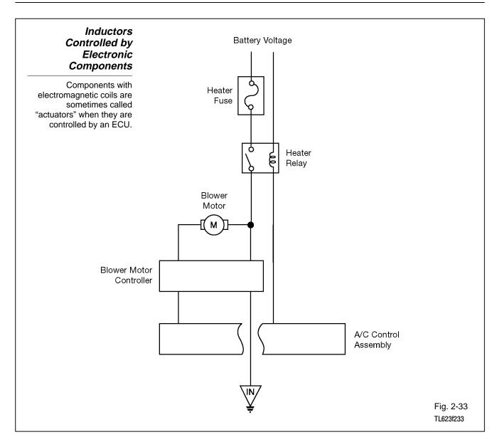
**Inductors controlled by electronic components -** Components with electromagnetic coils are sometimes called "actuators" when they are controlled by an Electronic Control Unit (ECU). Keep these things in mind when dealing with actuators:
