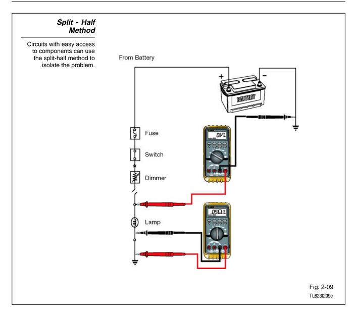
**Split-Half Method** - You can use the split-half method on circuits where access to the related components is good. The split-half method works as follows:
