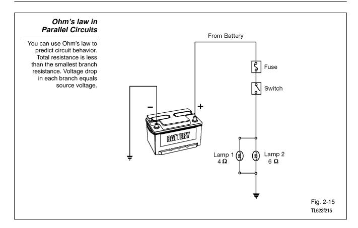
**Applying Ohm's Law** - You can use Ohm's Law to predict the behavior of electricity in a circuit.
