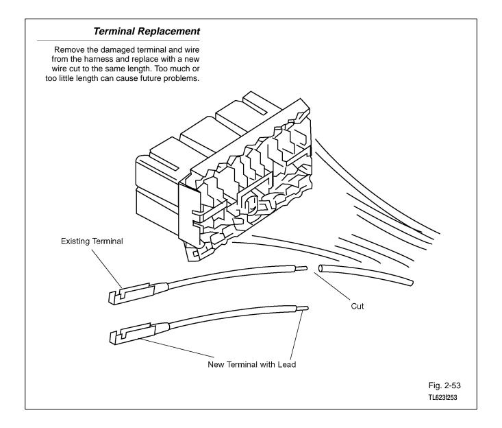
7. Strip insulation from wire on the harness and replacement terminal lead.
