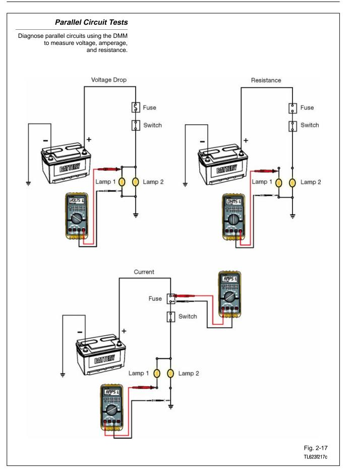
**Parallel circuit tests** - Use these guidelines to measure current, voltage, and resistance in parallel circuits:
