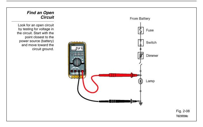
**Testing for available voltage -** Find the fault in an open circuit by testing for available voltage.
