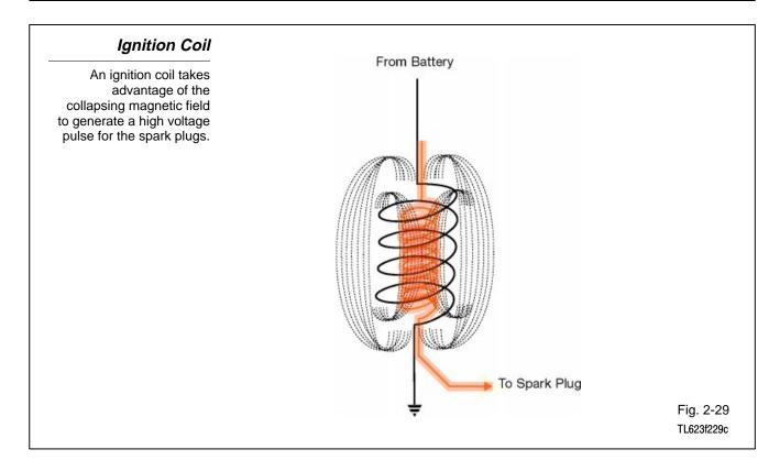
Ignition coil - An ignition coil is one type of inductor.
