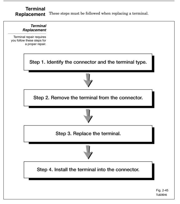
Step 1. Identify the connector and terminal type.
