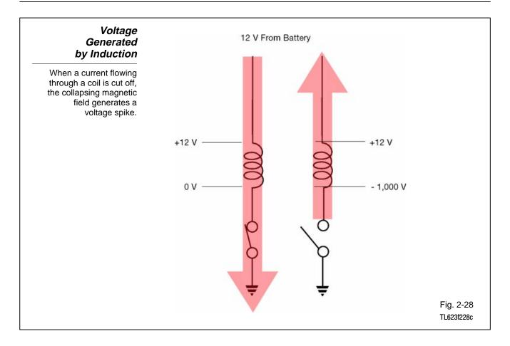
**Inductor coil control devices -** These control devices can turn coils on and off as needed to control solenoids and relays:
