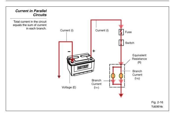
**Current** - Current in a parallel circuit behaves differently than it does in a series circuit.
