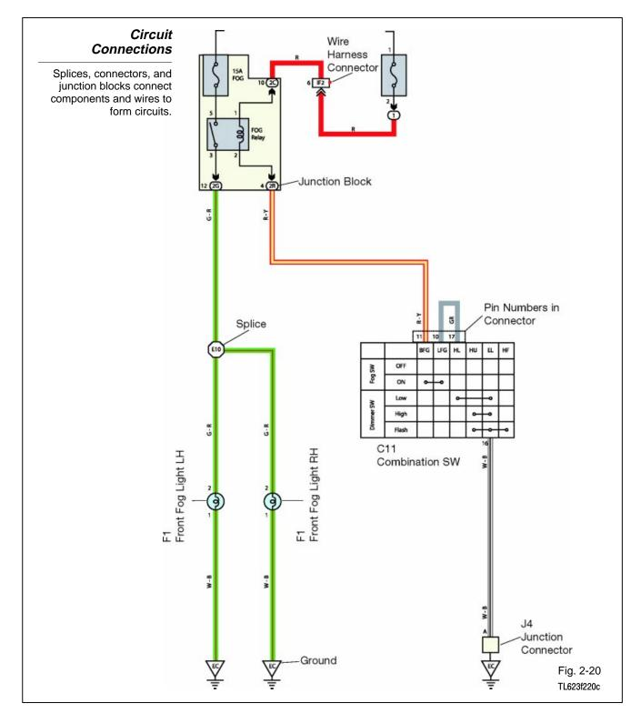
Load Control Switching devices control current in circuits: Source or Ground • Relays
