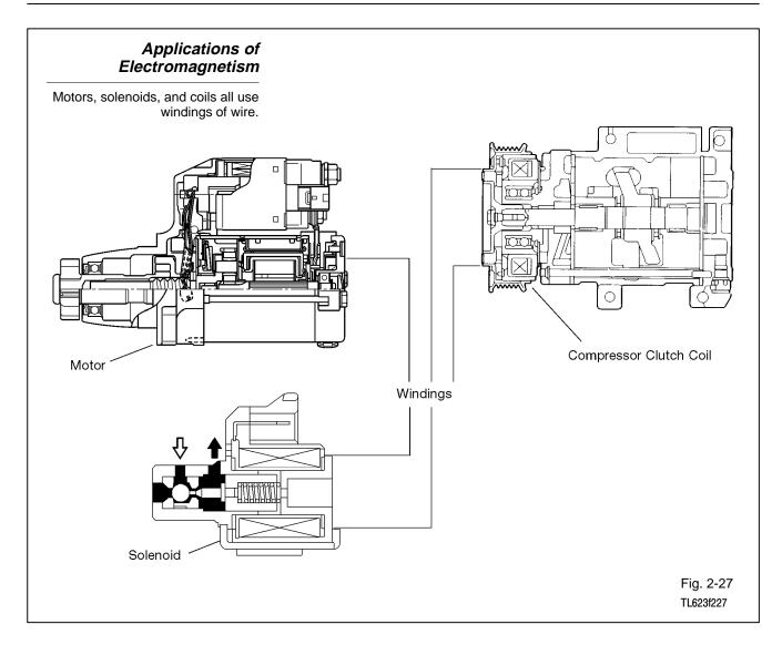
**Applications of electromagnetism -** Automotive electrical systems use electromagnetism in various ways:
