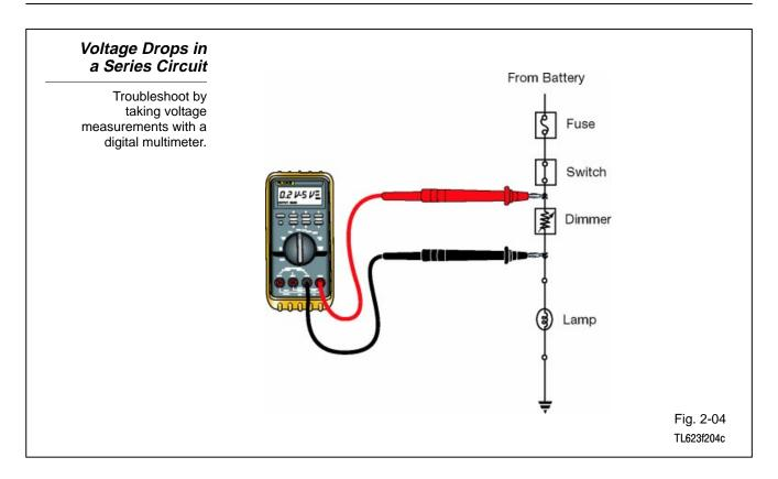
**Voltage drops in a series circuit** - Every element in a circuit that has resistance generates a voltage drop.
