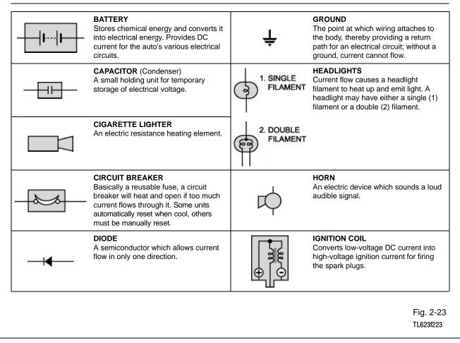
Standardized electrical symbols allow wiring diagrams to efficiently convey information about automotive electrical and electronic circuits.
