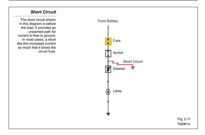
**Short circuit** - A short circuit is a fault in the current path. A short can be:
