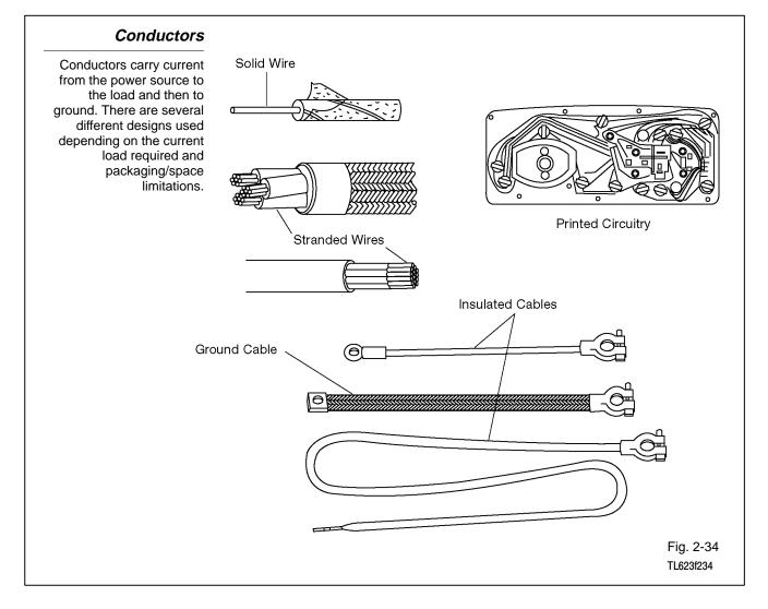
**Conductors** Conductors allow electrical current to flow from the power source to the working devices and back to the power source.
