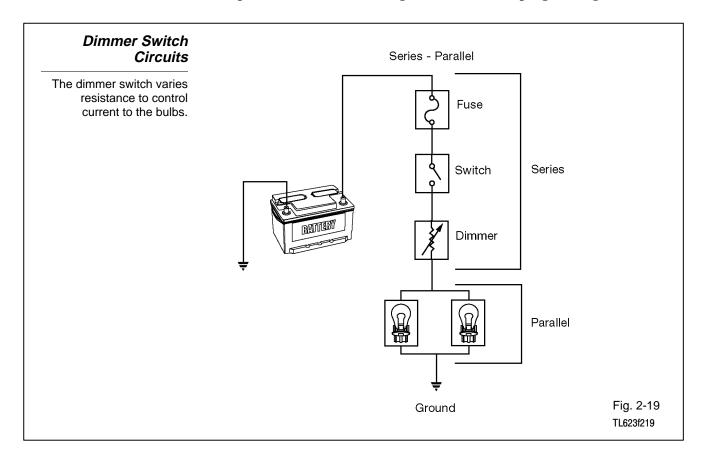
**Circuit connections -** Various devices connect components in series and parallel segments:
