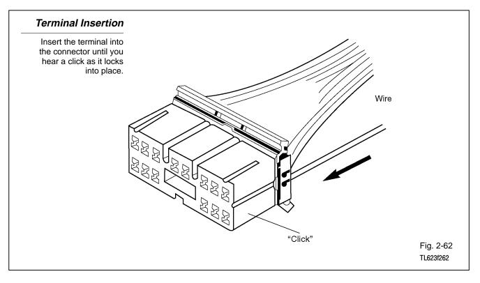
a) When properly installed, pulling gently on the wire lead will prove the terminal is locked in the connector.
