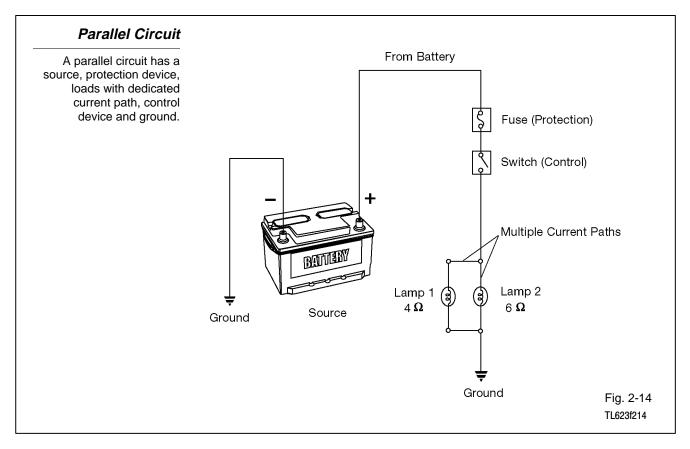
A parallel circuit contains all the elements of a series circuit:
