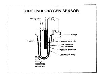
charged oxygen ions form on the platinum plates. The amount of oxygen to which each plate is exposed determines how many ions form on the plates. When there is a difference in the number of ions on the plates, a difference in potential or voltage occurs between the two plates. The less oxygen there is in the exhaust, the greater the voltage produced. When the air-fuel mixture is lean, the voltage created is low. Conversely, when the mixture is rich, the voltage is high.
