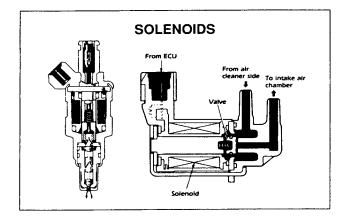
Solenoids are controlled two ways: pulse width or duty cycle. Pulse width control is used when the frequency is not consistent. An example of pulse width is a fuel injector which is turned on for a determined length of time and then shut off. Duty cycle control is used when the frequency does remain constant. A duty cycle solenoid in ABS is designed to be on and off for a specific time according to a selected ratio-on for 20% of the time and off the other 80%.
