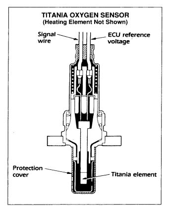
sensor is at operating temperature, the amount of oxygen to which the titania is exposed. will change the physical resistance of the sensor. The ECU supplies a reference voltage to the sensor and monitors the voltage at the signal wire, similar to a thermistor.
