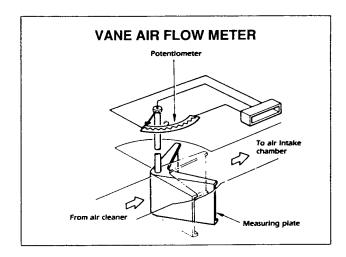
The vane type air flow meter on an EFI equipped vehicle is a common location on a Toyota for a sensor that uses a potentiometer. This sensor converts the air flow meter vane opening angle to a voltage and sends it to the Electronic Control Unit (ECU). This signal allows the ECU to determine the volume of air that is entering the engine.
