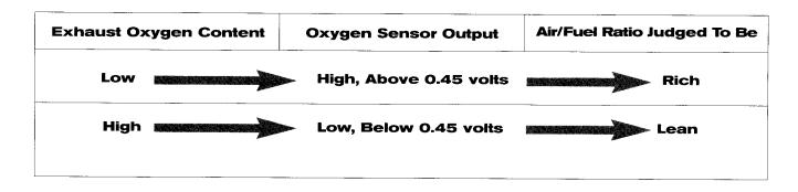
From the oxygen content, the ECM can determine if the air/fuel ratio is rich or lean and adjusts the fuel mixture accordingly. A rich mixture consumes nearly all the oxygen, so the voltage signal is high, in the range of 0.6 - 1.0 volts. A lean mixture has more available oxygen after combustion than a rich mixture, so the voltage signal is low, 0.4 - 0.1 volts. At the stoichiometric air/fuel ratio (14.7: 1), oxygen sensor voltage output is approximately 0.45 volts.
