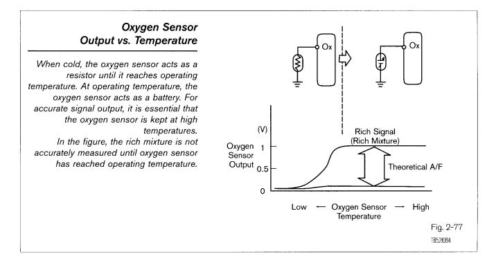
The oxygen sensor will only generate an accurate signal when it has reached a minimum operating temperature of 400'C (7500F). To quickly warm up the oxygen sensor and to keep it hot at idle and light load conditions, the oxygen sensor has a heater built into it. This heater is controlled by the ECM. See Oxygen Sensor Heater Control for more information.
