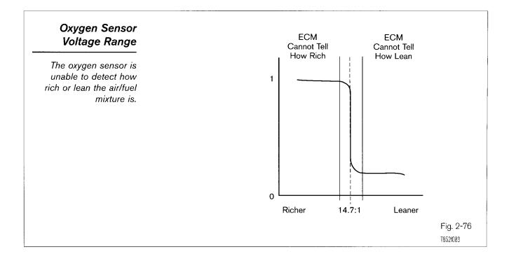
Small changes in the air/fuel ratio from the stoichiometric point radically changes the voltage signal. This type of oxygen sensor is sometimes referred to as a narrow range sensor because it cannot detect the small changes in the exhaust stream oxygen content produced by changes in the air/fuel mixture. The ECM will continuously add and subtract fuel producing a rich/lean cycle. Refer to Closed Loop Fuel Control in the Fuel Injection section for more information.
