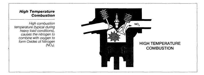
Generally speaking, the largest amount of NOx is produced during moderate to heavy load conditions when combustion pressures and temperatures are their highest. However, small amounts of NOx can also be produced during cruise and light load, light throttle operation. Common causes of excessive NOx include faulty EGR system operation, lean air/fuel mixture, high temperature intake air, overheated engine, excessive spark advance, etc.
