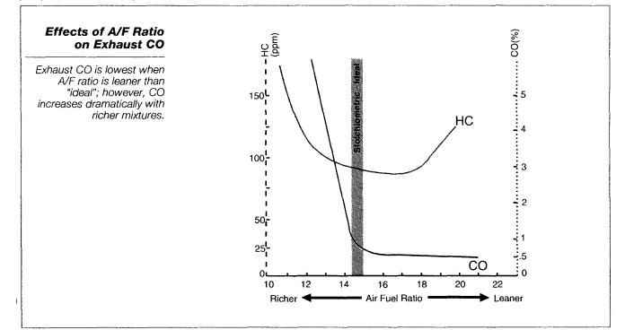
When the engine is at warm idle or cruise, very little carbon monoxide is produced because there is sufficient oxygen available during combustion to fully oxidize the carbon atoms. This results in higher levels of carbon dioxide (CO2) the principal by-product of efficient combustion.
