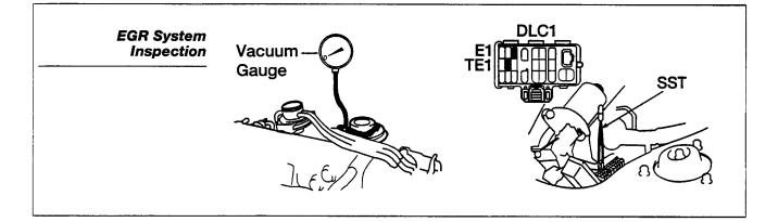
• With coolant temperature cold (A/T: below 140' F, M/T: below 131' F) and engine at 2500 rpm, the vacuum gauge should indicate zero.
