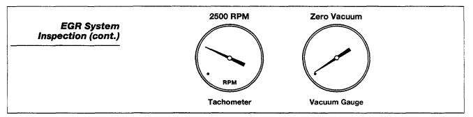
• Next, warm the engine to operating temperature and maintain 2500 rpm. The vacuum gauge should now indicate low vacuum (typically around 3")
