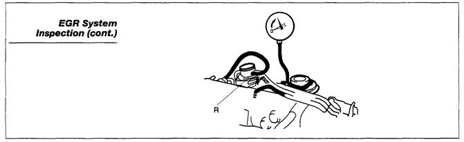
• Disconnect terminals TE1 and EI at DLC1 and reattach the EGR hoses to their original location.
