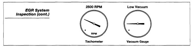
Next, with engine speed at 2500 rpm, connect the R port of the EGR modulator directly to a manifold vacuum source. The vacuum gauge should now indicate high vacuum (typically around 13") and the engine should run rough.
